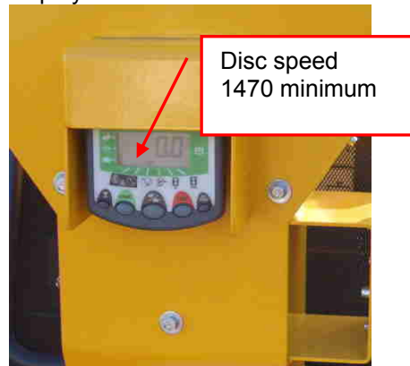
Fig 5.4 RDS Control unit display.
