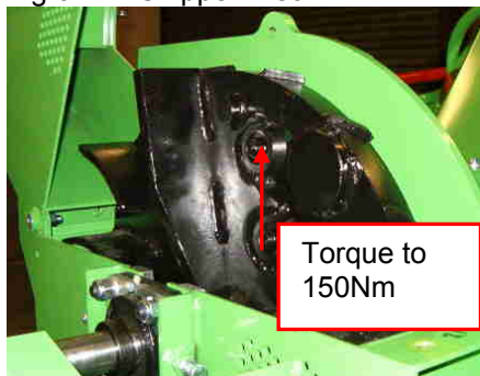
Fig 6.7.1 Chipper Disc
