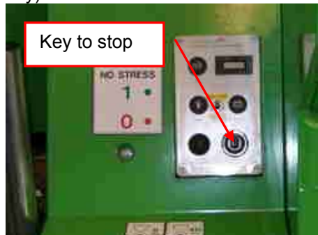
Fig 3.4.2 Engine Stop Switch - (start key)
