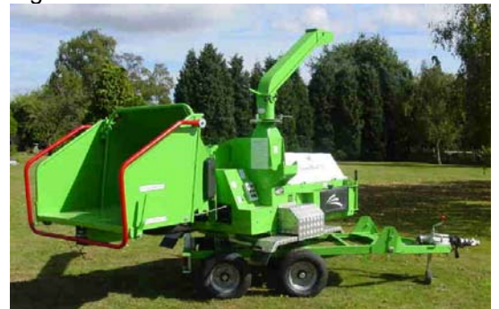
Fig 2.3 360 CM220MT55-360 with turntable
